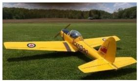
The plans include 6 sheets 36" x 80" with all parts and patterns shown. A cowl and canopy are available. Undercarriage is 5/8" diameter Robart Robo-Struts. The wing is two-piece, plug-in type with the wing break just outside of the wing walk so the wing to fuselage fairings are constructed as part of the fuselage.
